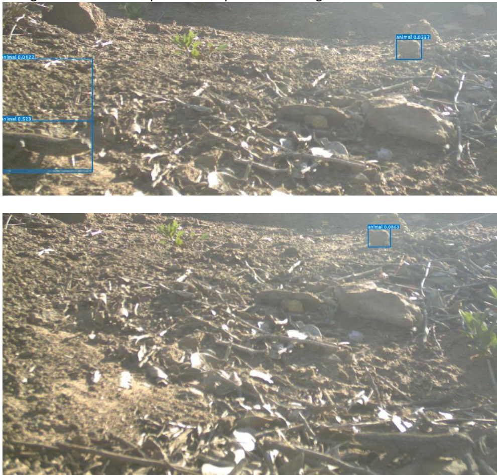
Figure 75 False positive and negative detections using Megadetector
