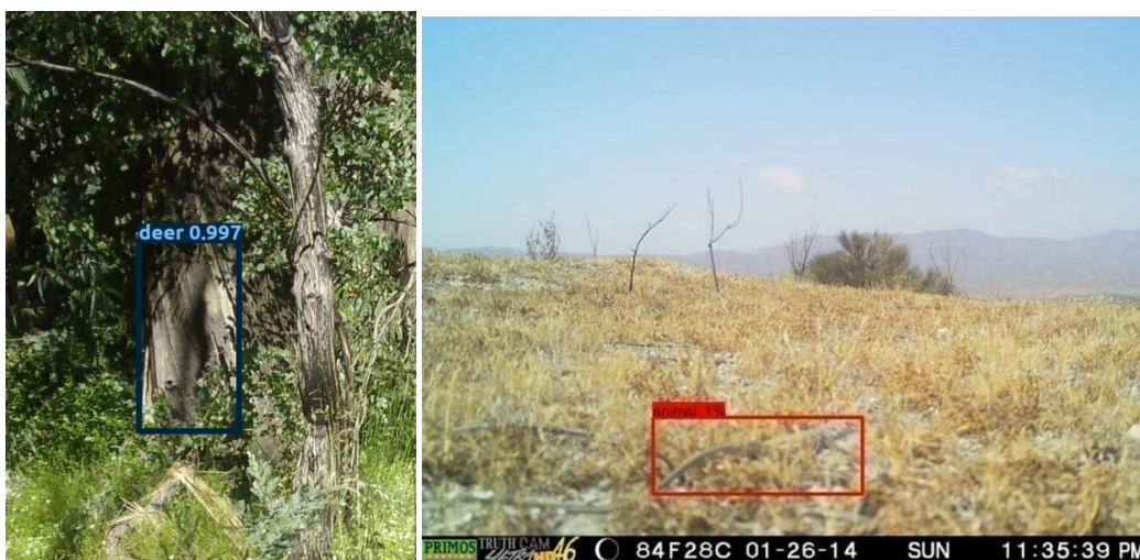
Figure 121 High-confidence spurious detection (left) and low-confidence detection of camouflaged lizard (right)
